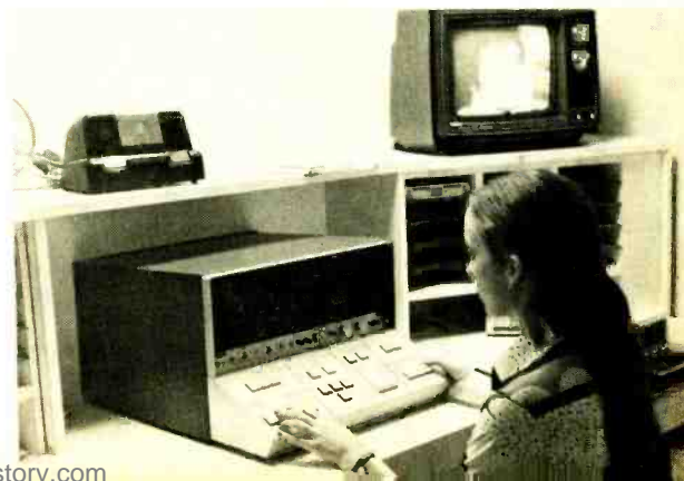
Young editor compiling a decision list using a Datatron 5050 editing system. Master cassettes can be processed through a CVS 504 TBC and be used directly on-air.
