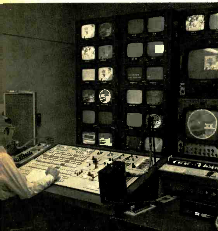
Engineer at control station setting up a microwave loop with the WTVJ remote ENG van.
