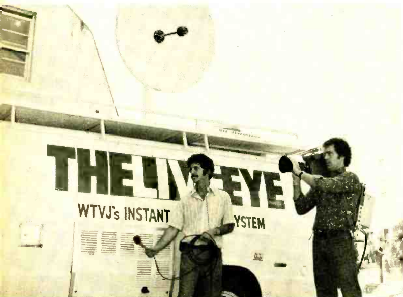
The WTVJ remote van prowls the Miami coastline with its Ikegami cameras, Sony 3800 VTR's and Microwave Associates dish. Signals can be transmitted to the main studios or to their Ft. Lauderdale transmitting facility.
