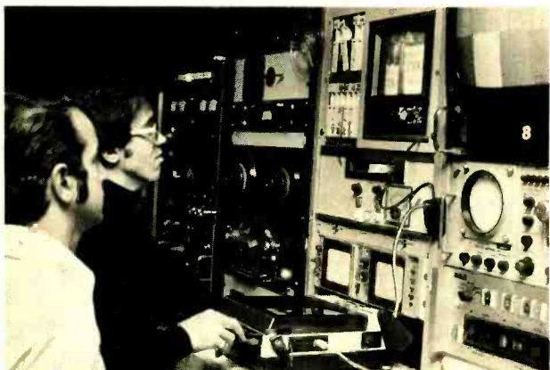
Ron Gerrilini (left) and Bob Hennessey transfer quarter-inch VTR to two-inch master tape for final editing before it is put on the air.
