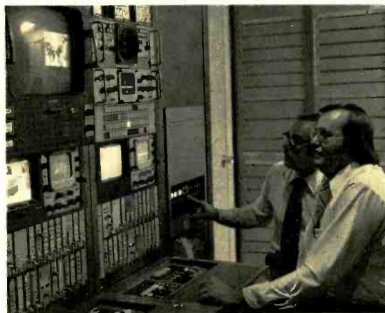
Joe Kline (left) and Bob Stone programming the CVS 600 synchronizer. Compression function is clearly shown in the monitors. Operator has a choice of six quad positions, one of the automatic positions can be reprogrammed for any "wild card" location.
